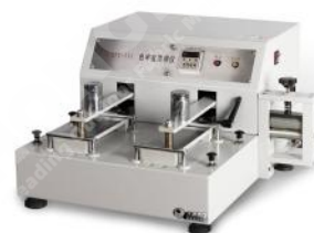
Friction Color Fastness Tester 摩擦色牢度仪
